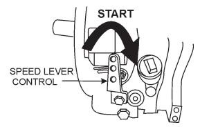
Figure 8. Engine Speed Lever (START position)
